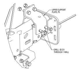
**5.** Remove and discard the two sway-bar bracket bolts and nut-clips from the sway-bar bracket (05-07 models).
