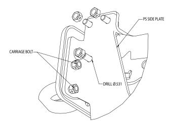
**4.** Attach the Upper Support Plate to the Side Plate [PS] (4) with two bolts (15). Using this item as template, drill two holes diameter 0.531" and fasten them with two locknuts (16).
