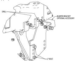
**10.** Install the bumper mounting bracket as shown using  $\frac{1}{2}$  -13 x 1.5" bolts & the special welded bolts w/ handle (12).
