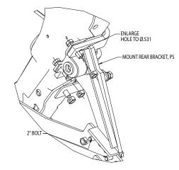
**9.** Hold the Mount rear bracket onto the frame and use it as a template to drill 2 holes 0.531". Install the ½"-13 x 1.5 bolts with lock nuts in the appropriate location.
