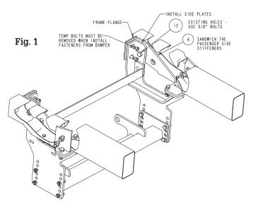
**4.** Install the additional rear Support Bracket (7) onto the rear of the frame. Secure the Bracket through an existing hole through the frame with one 5/8- $11 \times 2$ " bolt (11) and a nut (15). Drill the upper holes as needed and secure it with another 5/8- $11 \times 2$ " bolt and nut.
