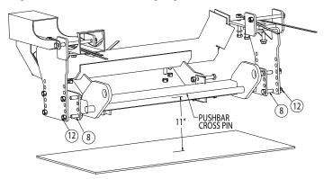
11. Install the CEN-SUPPORT BRACKET (4) to the push bar using four ½-13 bolts (8) and four locknuts (12). By holding up the part to the cross-member beam, drill out four 9/16" holes (if not already exist). Use the four ½-13 BOLT WITH HANDLES (13) and four locknuts to secure it onto the beam. You may have to loosen all fasteners in order to attach them.
