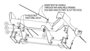
**12.** Torque all fasteners as shown in the chart. Check and re-torque all fasteners after 5 hours of usage to ensure safe plow operation. Ensure all coolant lines and wires are clear of moving or hot components and tie up as necessary.
