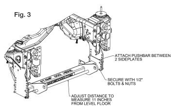
**6.** Temporarily, lower the swaybar from the bottom of the truck. Install the Swaybar Bracket (4) and re-attach the swaybar into place like a sandwich. Make sure to insert the Swaybar Spacer (6) up against the rubber toward the frame. Secure it with two new metric bolts (10). Connect the Rear Brace (5) to the Pushbar (3) and the Swaybar Bracket (4). Loosely, secure them together with four 1/2" fasteners.
