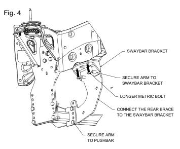
7. Repeat Step number 6 for the PS Rear Brace Arm (4).8. Torque all fasteners as shown in the chart. Check and re-torque all fasteners after 5 hours of usage to ensure safe plow operation. Ensure all coolant lines and wires are clear from moving or hot components.
