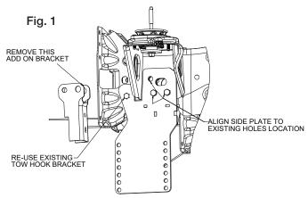
**3.** At the bottom of the sideplate, mark and drill open one hole from the frame and install one 1/2" bolt and nut. A nut on a stick is provided to help maneuver the bolt alignment. This stick may have to be bent and twisted in order to match the holes you just drilled.
