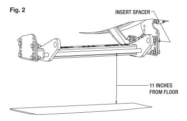
**5.** Install the PS Rear Brace (3) onto the Pushbar (2) using two 5/8" bolts and nuts. Secure the back of the bracket onto the back part of the Frame aligning to the bottom metric bolts. Reuse the existing nuts to secure it to the frame. Attach two more 5/8" bolts to the frame of the truck using the existing holes of the truck. For some early models, it is necessary to drill the two holes here. Secure them with two 5/8" nuts.
