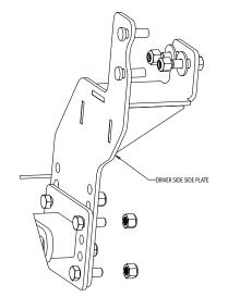
**5.** Mount the **PUSHBAR** (1) in place between the two side plates using eight ½"-**13x1-1/2" BOLTS** (5) and eight ½"-**13 LOCK NUTS** (8). The centerline of the Pushbar Crosspin should be approximately 9" to 10" from the ground. The air dam of the vehicle may need to be altered to accommodate this height. Improper mounting height will result in uneven cutting edge wear.
