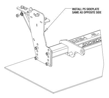
**5.** Assemble the Pushbar (3) between two Side Plates using eight 1/2" x 1.5" bolts provided. Adjust the Push Bar up and down. The center line of the push bar Cross Pin should be approximately 9" to 10" from the level ground. The plastic extension from the bumper/air deflector may need to be removed or modified.
