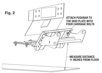
**5.** Torque all fasteners as shown in the chart. Check and re-torque all fasteners after 5 hours of usage to ensure safe plow operation.
