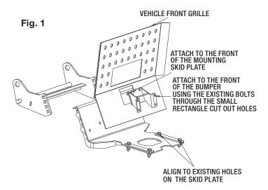
**3.** Look to the center front grille of the vehicle with a rectangular cut-out hole, and install the center bracket with four existing bolt holes onto front bumper bracket. Next, attach the bracket to the front of the mounting skid plate (1) with the three carriage bolts (4) and three nuts (6), and washers (5).
