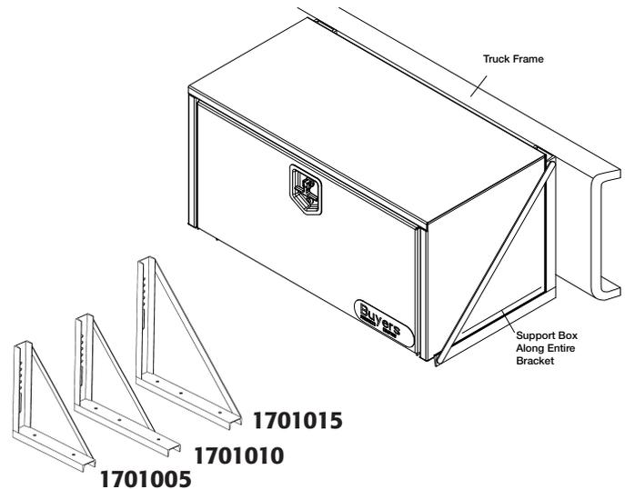
To properly support your Underbody Toolbox, we recommend the use of bottom support mounting brackets. These brackets should be placed so that each end of the toolbox is supported by the full width of the mounting bracket. To prevent rust, touch-up drilled holes with aerosol paint. To prevent water leaks, apply silicone sealant all around each fastener after installation.
