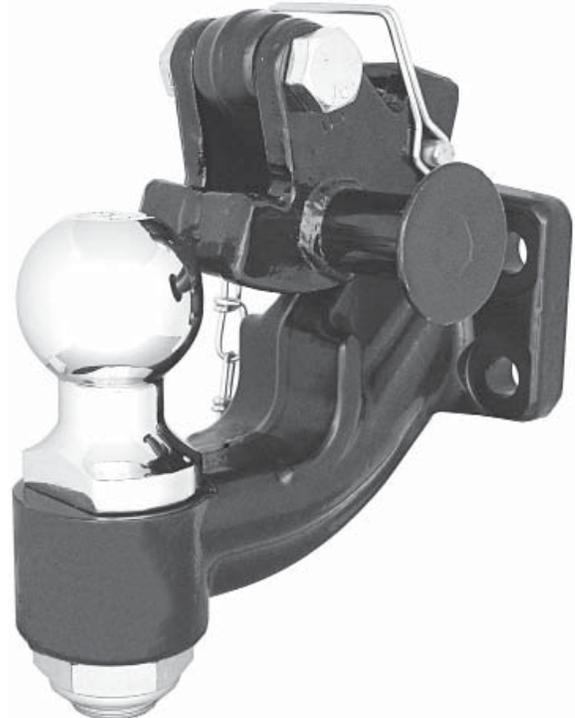
4. To close latch, pull plunger, rotate latch closed and release plunger. Plunger must be fully engaged to lock the latch. Assembly safety pin.
