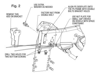
**4.** Look to the bottom of Fig 2, drill out two 1/2 inch holes to allow the 1/2 bolt installation from the bottom. Secure it with the nut on a stick and some washers. The stick may have to be bent and twisted in order to match the holes you just drilled.
