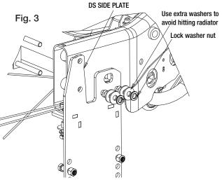
**6.** Assemble the Pushbar between two Side Plates using eight 1.5" bolts provided. Adjust the push Bar up and down. The center line of the push bar Cross Pin should be approximately 9" to 10" from the level ground. The plastic extension from the bumper/air deflector may need to be removed or modified.
