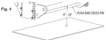
**7.** Lower the swaybar from the bottom of the truck temporarily. Install the Swaybar Bracket (5) and re-attach the swaybar into place like a sandwich. Make sure to insert the Swaybar Spacer (18) up against the rubber toward the frame. Secure it with two new metric bolts (15). Connect the Rear Brace (1) to the Pushbar (2) and the Swaybar Bracket (5). Loosely, secure them together with four 1/2" fasteners. (see Fig 5)
