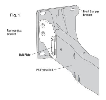
**3.** Remove the nuts from the PS Bolt Plate. Install the PS Side Plate onto the double bolts. Reinstall the two nuts just removed earlier. Install the long bolts (PN 3005140) provided in the lower holes. Secure these with the 1/2 fasteners provided. Diesel vehicle may require thin spacers nut to avoid interference (see Fig. 2).
