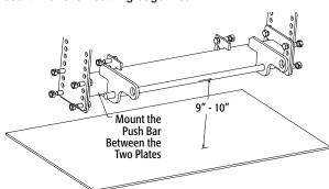
**3.** Look to the side of the PS Side Plate (2), drill through one wall with Ø.531 drill. Insert one Bolts with Handle (6) along with two Washers (7 & 10) and secure them with one ½" Nut (9) through the slot hole. Secure the other drilled-hole with one Bolt with Handle (6) and one ½" Nut (9).
