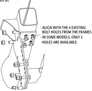
**5.** Mount the Pushbar (1) in place between the two side plates using eight  $\frac{1}{2}$ -13 x 1.5 bolts (8) and eight  $\frac{1}{2}$ -13 locknuts (9). The centerline of the Pushbar cross pin should be approximately 9" to 10" from the ground. The air dam of the vehicle may need to be altered to accommodate this height. Improper mounting height will result in uneven cutting edge wear.
