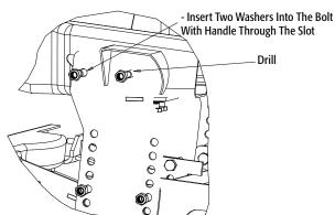
**6.** Position the PS Rear Brace (4) to the frame and secure it onto the Pushbar (1) with two ½-13 fasteners (8 & 9). In the back, secure the Rear Brace to the truck's cross member frame using two 3/8" bolts (11) and two 3/8" nuts (12). You may have to enlarge the hole to fit it through.
