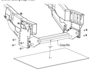
**5.** Position the PS Rear Brace (2) to the frame and secure it onto the Pushbar (1) with two ½-13 fasteners (11 & 12). In the back, secure the Rear Brace to the truck-frame using one 5/8-11 x 5 bolt (7) and one 5/8" nuts (8). You may have to enlarge the hole to fit it through.
