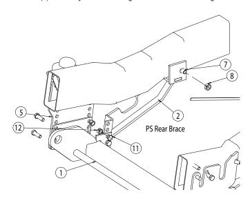
**6.** Position the DS Rear Brace (3) to the frame and secure it onto the Pushbar (1) with two  $\frac{1}{2}$ -13 fasteners (11 & 12). Look to the back of the Rear Brace (3), and temporarily install the U-bolt (9) onto the frame. Mark and drill the two holes  $\emptyset$ .531" through one wall. Undo the U-bolts and insert the bolt-sticks (6) through the newly drilled holes. Finally, re-insert the U-bolt and secure the Rear Brace (3) to the truck-frame with proper nuts and a spacer (10).
