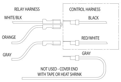
Instructions For Use With 16160100/B Relay Harness. Contact SnowDogg Tech Support At 866-974-3644 For Use With Earlier Harnesses.
