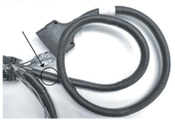
**5.** Pull the sheathing back on the harness away from the relay module and find the 2x GREEN and 2x YELLOW wires.
