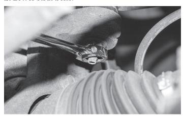
**c.** Upper ball joint nut - it may be separated by striking on the side with a mallet or hammer
