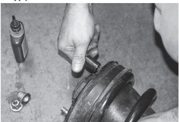
8. Install the lift spacer.
